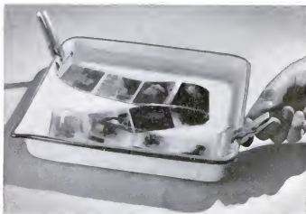
The strip of film is folded twice, and the ends are clipped to the tray with spring wooden clothespins
